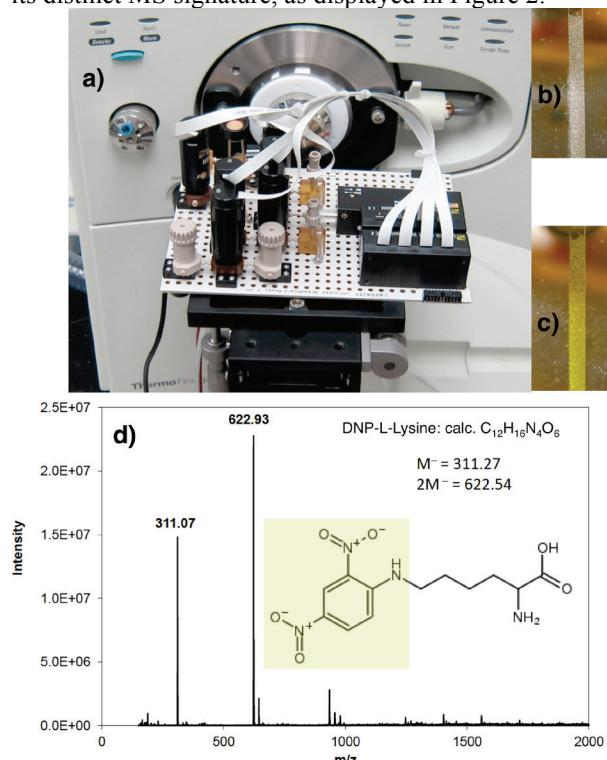
**Figure 2.** The above image a) displays a lab-on-a-breadboard mounted to a bench top MS to simulate a subsystem described by Science Tier 4. Highlighted are the 1-mm-wide microfluidic channels loaded with strong acid cation exchange resin beads before b) and after c) automated processing of a DNP-L-Lysine sample. Displayed in d) is the chemical structure, calculated and observed mass for detection by MS.
