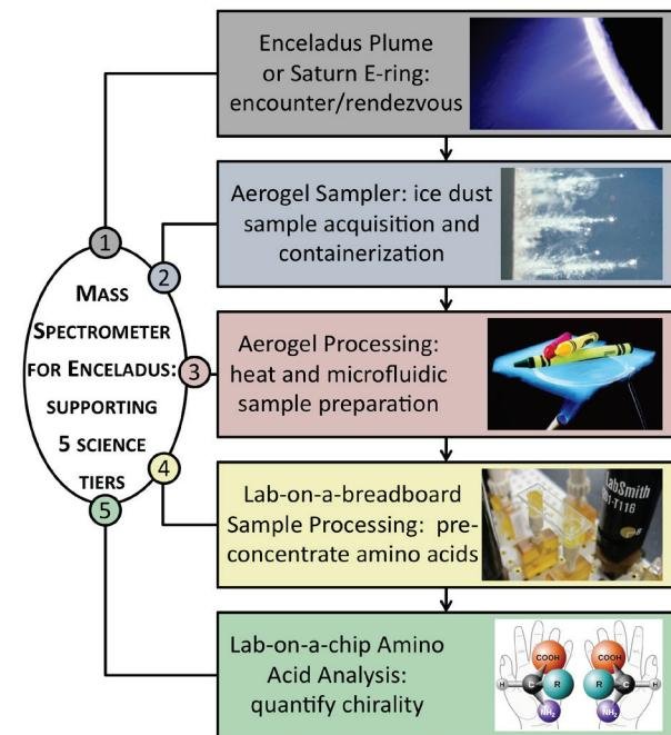
**Figure 1.** Arrows indicate the science instrument system operational sequence. The lines leading to the MS illustrate how the core subsystem is utilized during 5 stages of EAAS instrument operation, creating 5 distinct science tiers.
