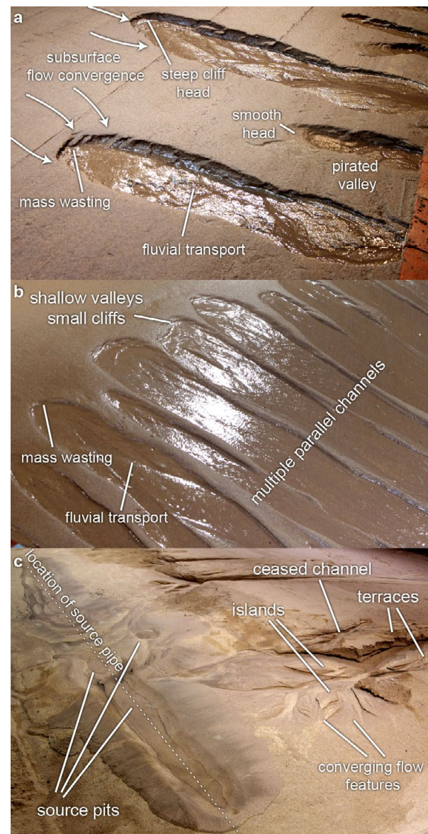
Fig. 1 Examples from the three types of experiments: a) regional groundwater source, in action; b) precipitation-fed seepage, in action; and c) pressurized groundwater (super-lithostatic), final dried morphology, subsurface source indicated. In all cases flow is from left to right.
