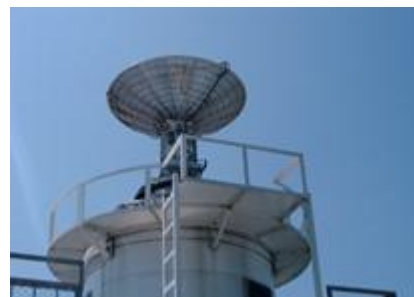
Fig. 2. A 2-m S-band antenna to be used for data downlink.
