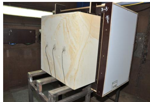
Figure 1. Rear surface of the sandstone target with mounted pressure gauges.
