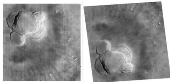
Figure 1. Viking image of the Olympus Mons caldera on Mars. The image on the left shows the raw PDS EDR and the image on the right shows the calibrated and map projected (orthorectified) science-ready image.
