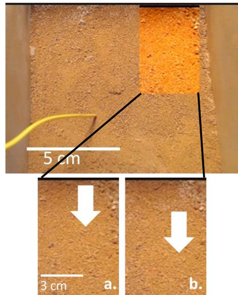
Fig. 3. Still images of regolith movement at 28° slope, 128 sec. apart. Arrows indicate positions of one sample grain.
