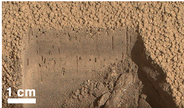
Figure 1. Sol 66 MAHLI image of horizons or banding in the wall of the first scoop trough at Rocknest.
