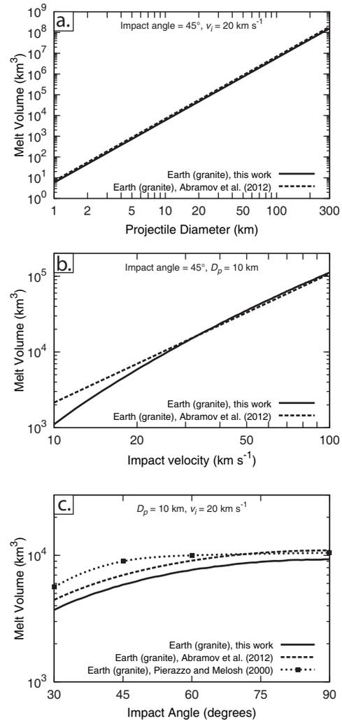
**Fig. 1.** Melt volume as a function of (a) projectile diameter, (b) impact velocity, and (c) impact angle. Effects of target temperature are not included here.
