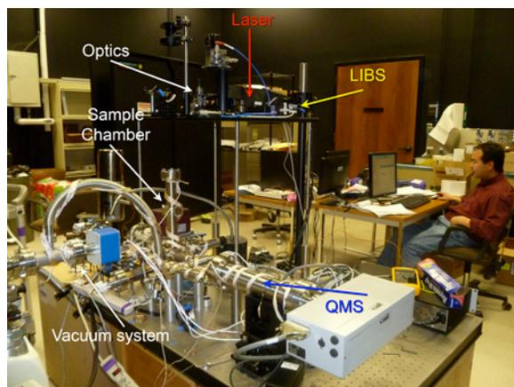
Fig. 1 KArLE breadboard, with integrated QMS and LIBS.
