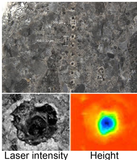
Fig. 4. (top) Optical image of a series of 10 LIBS ablation pits in Fish Canyon Tuff. (bottom) Concurrently measured laser return and depth profile (red=shallow; blue=deep) of Hole 7 (field of view  $\sim 500\mu\text{m}$ ).
