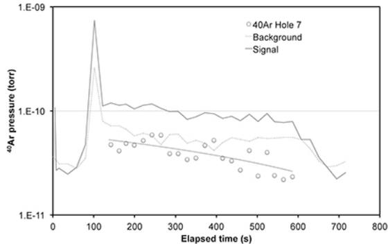
Fig. 3. QMS response at mass 40 to liberated gas from LIBS ablation. 300 LIBS shots were fired over 30 s at  $t=100$ s, causing the transient pressure spike. The data were extrapolated back to the abundance at  $t=100$ .
