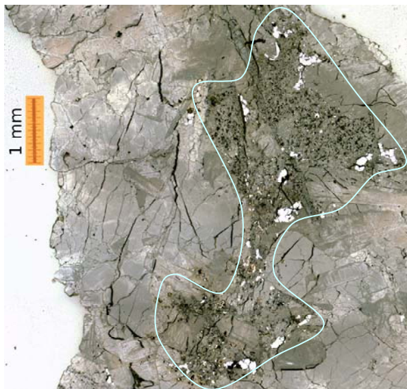
Figure 3: The large mesostasis region (outlined) in CMS 04049, 27 under reflected light. Note the large high reflectivity ilmenite grains and sulphides, making 0.7 modal %.
