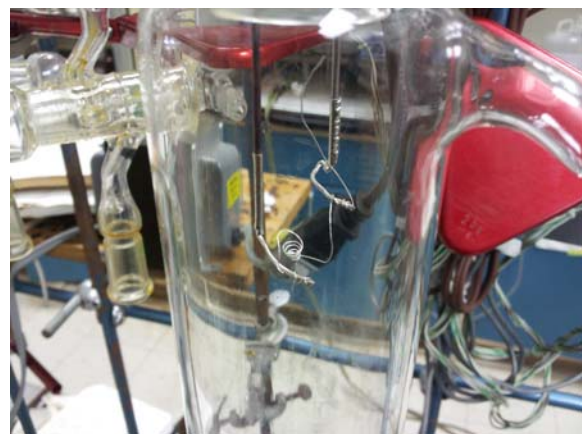
Fig. 3 Pt loop in glass vessel used for vaporization experiments. Pt resistance heater holds molten NaCl while vapor condenses on the glass walls chilled to liquid nitrogen temperature.
