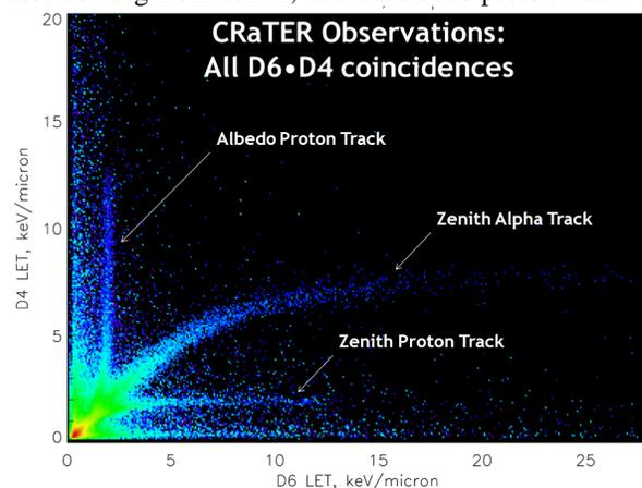
In this work, we use CRaTER observations to quantify the energy spectrum of this newly-discovered proton albedo. We use multiple-detector energy deposits of all those particles identified as proton albedo and invert these energy deposits to infer the incident proton albedo spectrum. This technique allows us to reconstruct the incident spectrum between ~65 and ~125 MeV.
