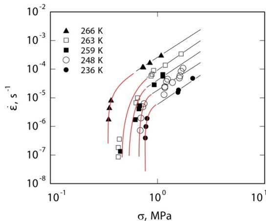
**Fig. 2** – Plot of strain rate vs. stress for ice containing 12 vol.% alumina of particle size  $0.3 \mu\text{m}$ . The slope of the straight line segments above  $\sim 1$  MPa is  $\sim n=2.4$ , in accord with expectations from the composite flow law of Goldsby and Kohlstedt [1] for  $d=1 \mu\text{m}$ . Red lines illustrate schematically the threshold stress-like behavior at low stresses. Note the temperature dependence of the threshold stress.
