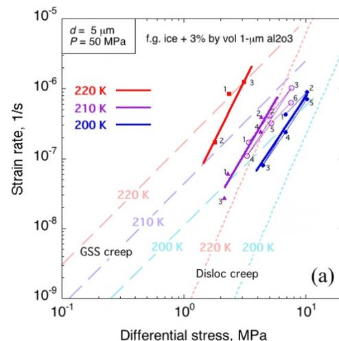
**Fig. 1** – Plot of strain rate vs. stress for ice containing 3 vol.% alumina of particle size 1  $\mu\text{m}$ . Numbers indicate the sequence of stresses at which strain rates were measured. Long-dashed lines show the flow law for GBS-limited creep [1] at each temperature; short dashed lines show the flow law for dislocation creep [2].
