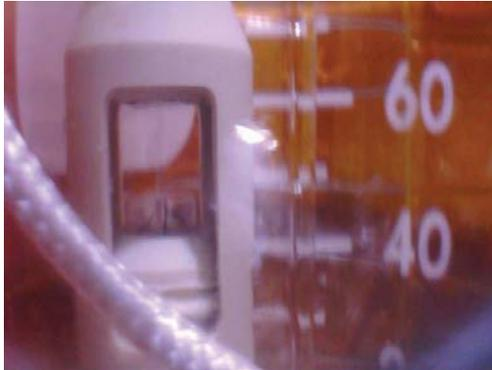
**Figure 3.** Endoscope view showing the optical path length of the fiber-optic UV-Vis probe immersed in ethane at 94 K. The white cable cutting across the view is for the temperature probe. Volume markings on the 150 mL beaker are visible.
