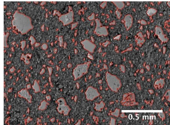
For the entire 4X3 region 1033 particles were defined. Once defined, a vast number of measures can be obtained for each particle. Following Rickman et al. [17] work on 6 simulants of the lunar regolith, results
