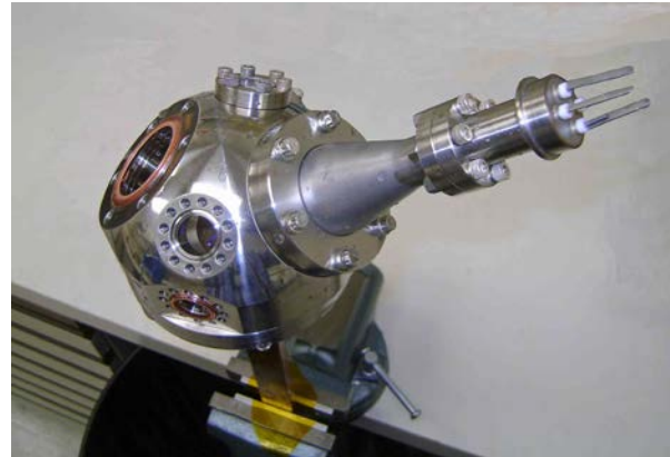
Figure 1: The sample chamber is shown after cleaning subsequent to the first charge of JSC-1A simulant. The two small open ports attach to the mass spectrometer and gas inlet manifolds. The larger open port attaches to the vacuum system. The vacuum feedthrough for the TCs is to the upper right.
