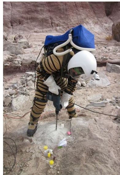
Figure 1: Rotary Percussive drilling while in suit. Note the cuttings around the hole.
