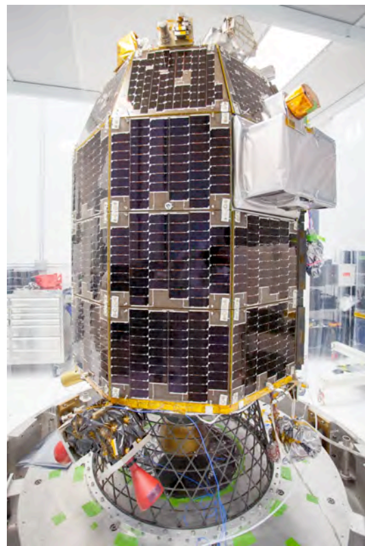
Fig. 1. LADEE in preparation for environmental testing. The neutral mass spectrometer is the large silver-colored box on the right. The lunar dust detector is at top right.
