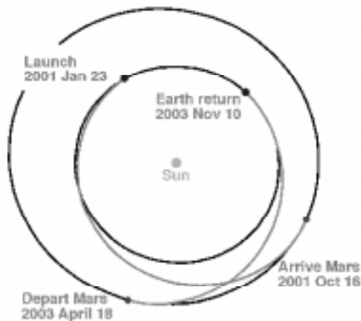
Fig. 1. Aladdin's orbit allows sample return from both Martian moons within three years after launch.
