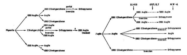
Fig. Ia. Schematic diagram outlining the exsolution and inversion phenomena in 67075, 18, 1 pigeonite.
