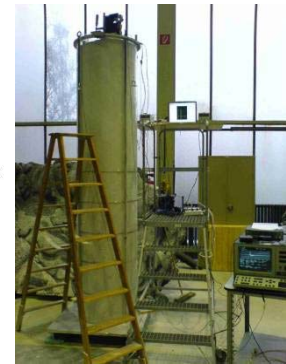
Figure 1: Schematics of the HP 3 instrument showing the functional subsystems (left); HP 3 Breadboard during 2.3 m soil intrusion test (right) – Support System is positioned at top of soil cylinder.
