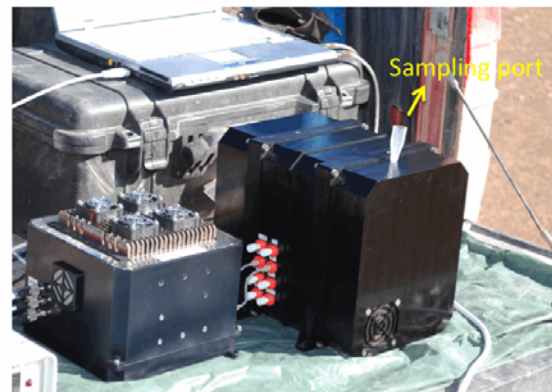
Fig. 2. The SOLID3 instrument in the field, showing its two functional units: the Sample Preparation Unit (SPU) (right) and the Sample Analysis Unit (SAU) (left). From ref. [7].
