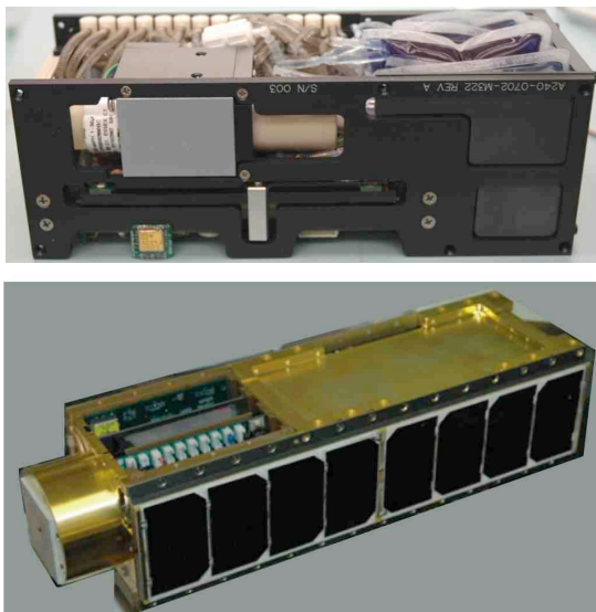
Figure 1. (Top) PharmaSat fluidic system prior to integration (~ 7x7x20 cm), including 2 pumps, a dozen active valves, 8 reagent and waste bags, and 48-well microfluidic card; (Bottom) Mostly-integrated PharmaSat. Spaceflight mass 5.1 kg; size 10x10x34 cm. This technology can be adapted to the measurement of Mars surface reactivity.
