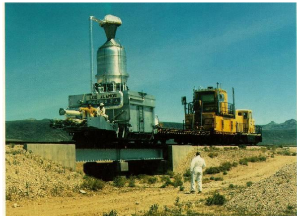
Figure 2. Phoebus-2A Nuclear Thermal Rocket en route to ground test (1968).
