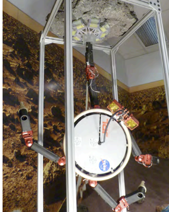
Figure 3 The LEMUR IIB robot hanging inverted off of a simulated cave ceiling using a microspine gripper.
