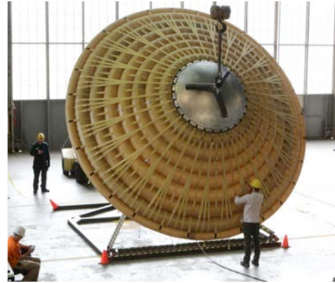
Figure 1: 6-m HIAD being readied for load and model correlation testing-ARC-NFAC (May/June 2012)
