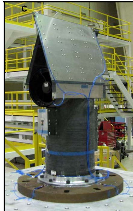
Fig. 2. The NanoEye structural test model, successfully vibration tested by ITT Exelis.
