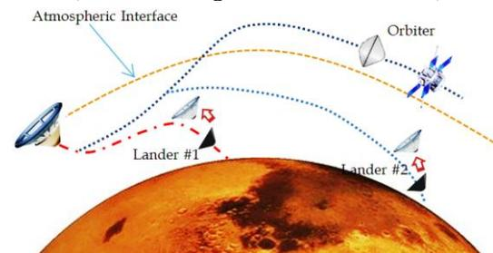
**Fig. 1: Dual-use ballute aerocapture concept. It is a combination of two elements (either both landers; or one lander and an orbiter). The IAD decelerates in the atmosphere. Element 2 jettisons and either land (lander #2) or exit the atmosphere (orbiter). The main system further descends with lander #1.**
