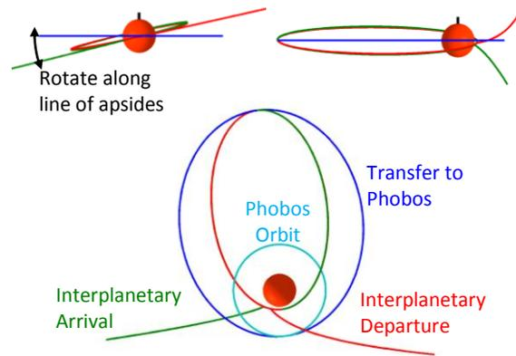
**Figure 4** Example transfer to Phobos.
