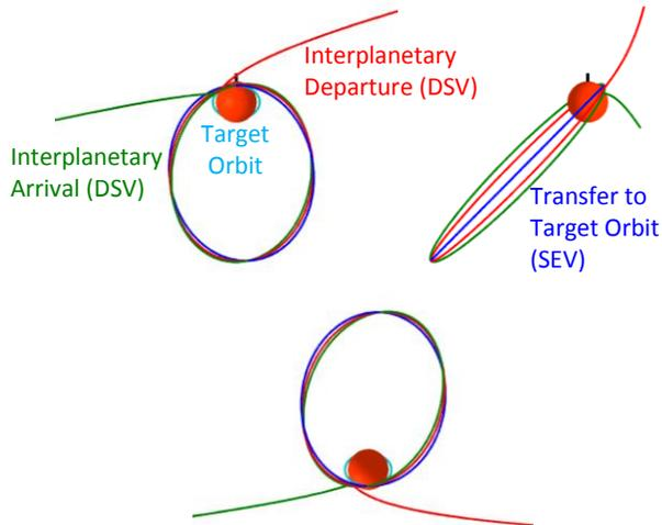
**Figure 2** Transfer from arrival interplanetary trajectory to a 500 km, 45 deg orbit, then to departure.
