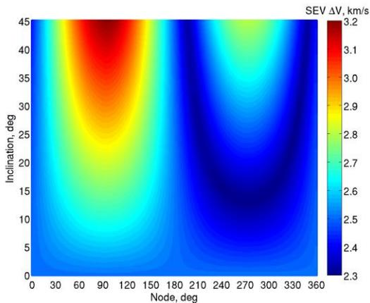
**Figure 3** Orbital transfer cost of the SEV to reach a variety of potential target orbits at 500 km altitude.
