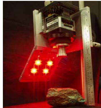
Fig. 1: Multispectral Microscopic Imager. Illuminator has 102 LED emitter dies; set of 4 emitting at 635 nm activated in this photograph; scale is marked in inches and cm.
