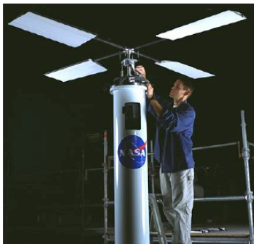
Figure 1: Test of conceptual Mars VTOL UAV rotor in NASA-Ames Mars Hover Chamber. Rotor is sized for \approx 10 kg UAV, is scalable to 50 kg UAV.
