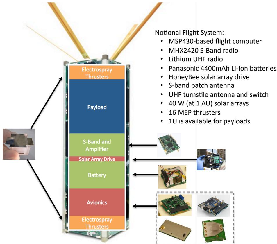
**Figure 2:** CubeSat and MEP technology could enable a 3-4 kg spacecraft capable of flight between Earth and Mars.
