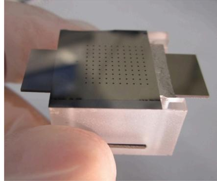
**Figure 1:** Prototype MEP thruster, feed system, and propellant - only 19x19x14 mm.
