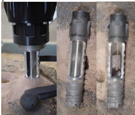
Figure 4. The PreView Bit. (L): after reaching the target depth, break-off tube is rotated to shear and capture the core. Once the tube is fully closed (C), the core cannot fall out. To view the core, the break-off tube is rotated back to expose it. (R)
