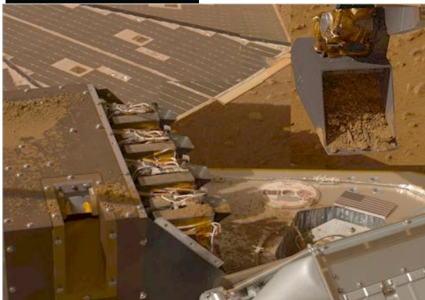
Figure 1. Left: one of four MECA Wet Chemistry Laboratory (WCL) cells flown on the Mars Phoenix Mission. Bottom: The MECA enclosure on Mars. Shown in the middle of the picture are the four WCL cells. In the foreground is the soil inlet for the microscopes.
