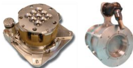
Fig. 1: Commercial propulsion systems approaching the capability needed for interplanetary flight of miniature spacecraft. Left, electro spray thruster from Busek with I_{sp}=1300 s. Right, ion thruster from Busek with I_{sp}=3800 s.
