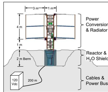
Figure 4. Simple, Deployable FSP System (10 kWe)
