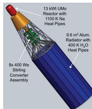
Figure 2. Kilopower System with Stirling (3 kWe)
