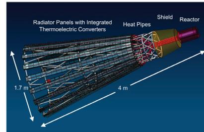
Figure 1. Kilopower System with TE (1 kWe)
