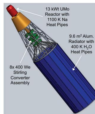
Figure 2. Kilopower System with Stirling (3 kWe)
