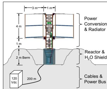
Figure 4. Simple, Deployable FSP System (10 kWe)
