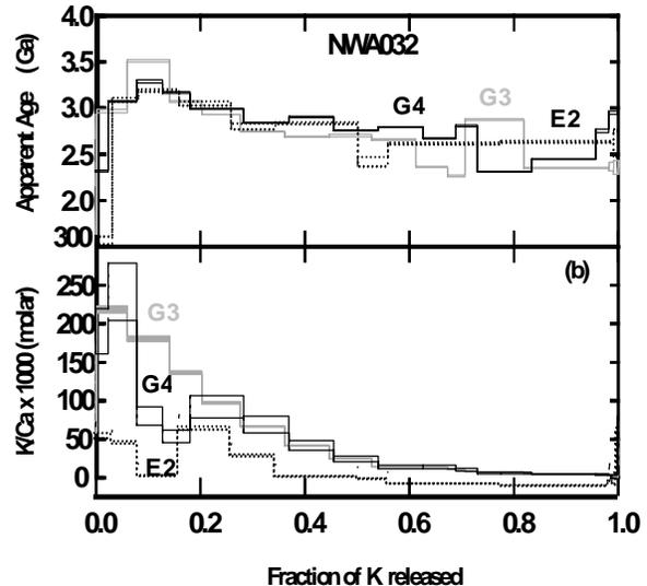
Fig.1 Ar-Ar step-heating results for samples G3, G4 and E2 of NWA 032: (a) Apparent ages and (b) K/Ca molar, vs Fraction K released.
