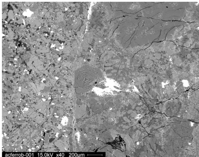
Backscattered electron image of NWA 5764: the LL6 lithology (left) and the L4 lithology (right) are separated by a  $\sim 20 \mu\text{m}$  vein filled with metal and sulfide.
