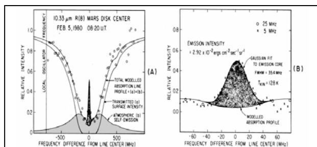
**Figure 1:** Infrared heterodyne spectra of Mars non-thermal emission with model, illustrating contributions to the observed spectrum. (A) Full line spectrum data at 25 MHz resolution and modeled components contributing to the observed spectrum: transmitted surface intensity, atmospheric LTE self-emission, and the narrow non-LTE emission core. (B) Non-LTE core measurement at 5 MHz resolution with fitted Gaussian function and retrieved kinetic temperature of 128 K.
