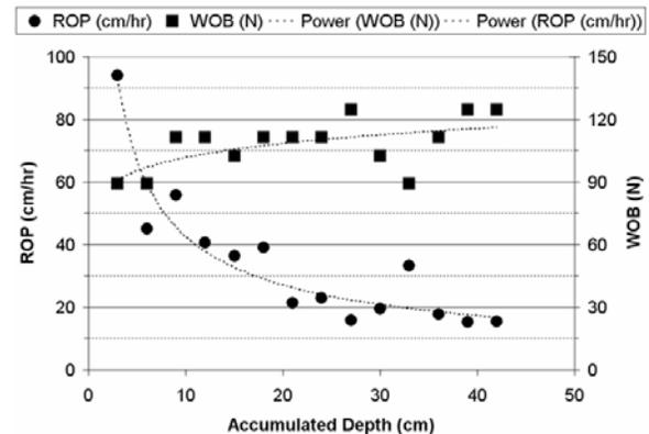
Figure 2. Rate of Penetration (ROP) and Weight on Bit (WOB) vs. Accumulated Depth for a single bit in 100 MPa Keweenaw Basalt. [2]
