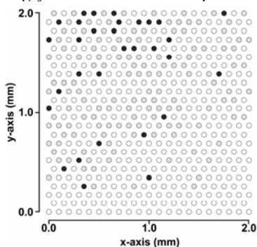
**Fig. 2.** Two-dimensional map showing heterogeneity of distribution of stearic acid biosignature in thenardite. Gray spots have m/z 390 peaks with S/N of 3 to 10 and black spots have S/N 10 or greater.
