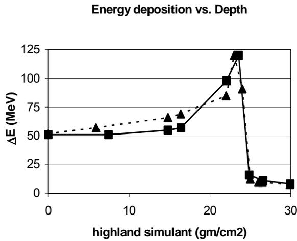
Figure 2. Average energy deposition of 290 MeV/nucleon <sup>10</sup>B ions in a 3mm silicon detector after passing through varying depths of lunar regolith simulant. Filled square: data with density correction; filled triangle: model.
