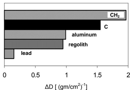
Figure 1. Average percent dose reduction per unit areal density (gm/cm<sup>2</sup>) for lunar regolith compared to polyethylene, graphite, aluminum and lead.
