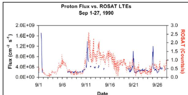
Fig.2. The correlation between the solar wind flux (blue solid) and the strength of the soft X-ray emission (red dashed).
