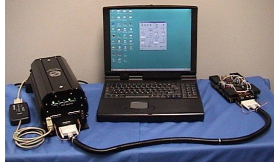
Figure 2. Electronics interface for fluidics controls and image acquisition. The dynamic microscopy platen is seen on the far right. The software environment provides users with opportunities to design, optimize and operate their experiments.
