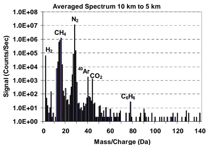
**Figure 2.** The direct inlet averaged mass spectrum from 10 km to 5 km showing the major atmospheric constituents of H<sub>2</sub>, CH<sub>4</sub>, N<sub>2</sub>, and <sup>40</sup>Ar. CO<sub>2</sub> may be due to background gas in the sensor.
