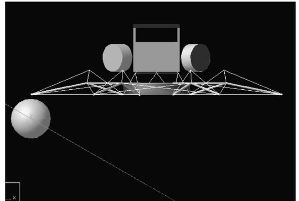
Figure 5: ADAMS simulation of pallet lander on a 30 degree slope with a 2 meter diameter rock half buried.
