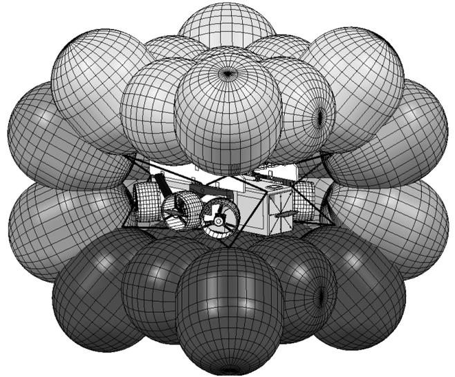
Figure 2: Isometric view of airbag landing system (2 bags removed for clarity).
