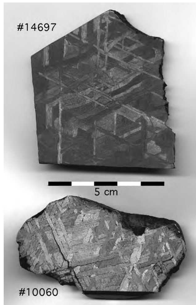
Fig. 4. Polished and etched surfaces of a IIIAB medium octahedrite (specimen #14697, 102.4 g) and a IAB coarse octahedrite (specimen #10060, 152.1 g) at Museo di Storia Naturale, Pisa University, previously reported as an unclassified iron meteorite of uncertain origin (Perchiazzi and Mellini 1995). Specimen #10060 is now identified as Toluca.
