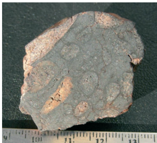
Fig. 3. Cut surface of NWA 5782 showing its brecciated texture. Units on scale (rule) are inches.
