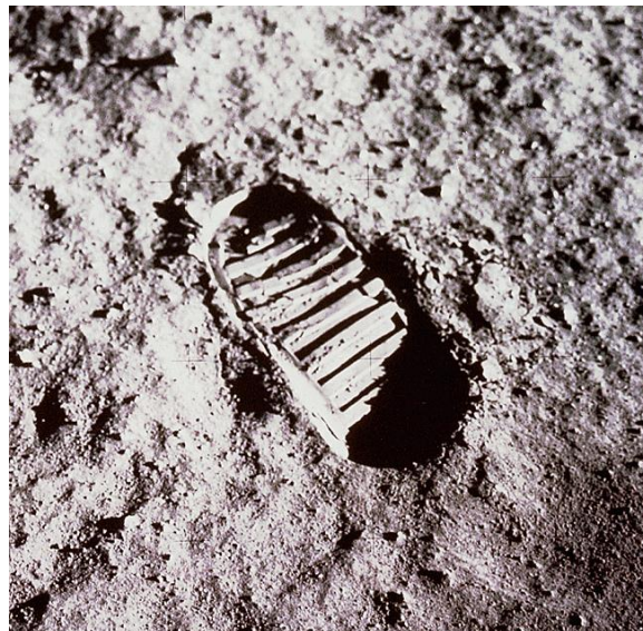
FIGURE 7.12 Apollo 11 astronaut Edwin “Buzz” Aldrin photographed this footprint in the lunar regolith. The photograph was part of an experiment to study the geotechnical properties of the Moon (specifically the effects of pressure applied to the surface). Image AS11-40-5878.
