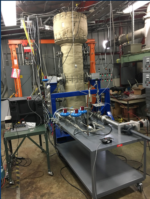
Drilling tests were performed under Venus conditions in the tall white chamber; pneumatic sample transfer hardware is on the table in the foreground
